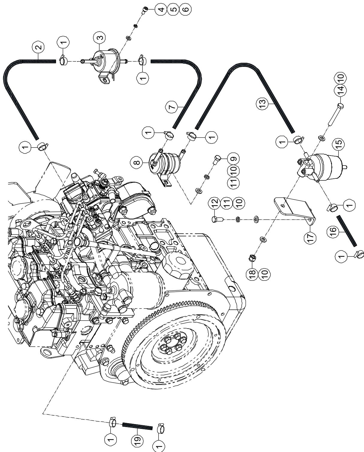
**1-25 Engine Fuel System Installations (Perkins Engine)**
