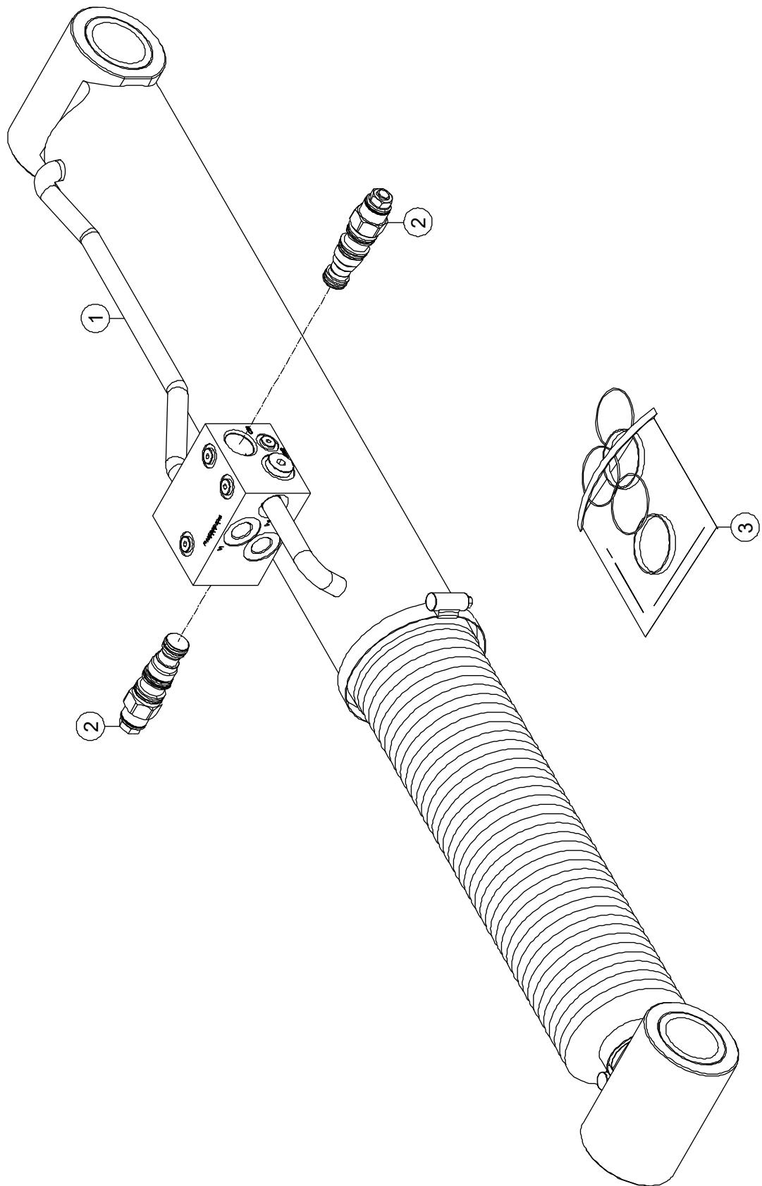
**5-6 JIB Leveling Cylinder Assembly**
