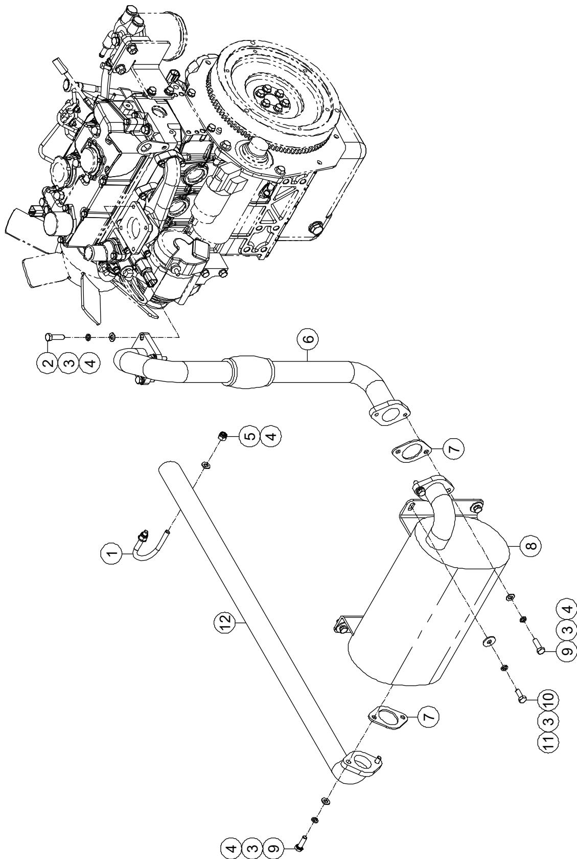
**1-29 Engine Exhaust System Installations (Perkins Engine)**
