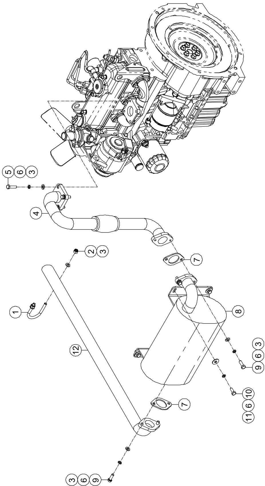
**1-28 Engine Exhaust System Installations (Kubota Engine)**
