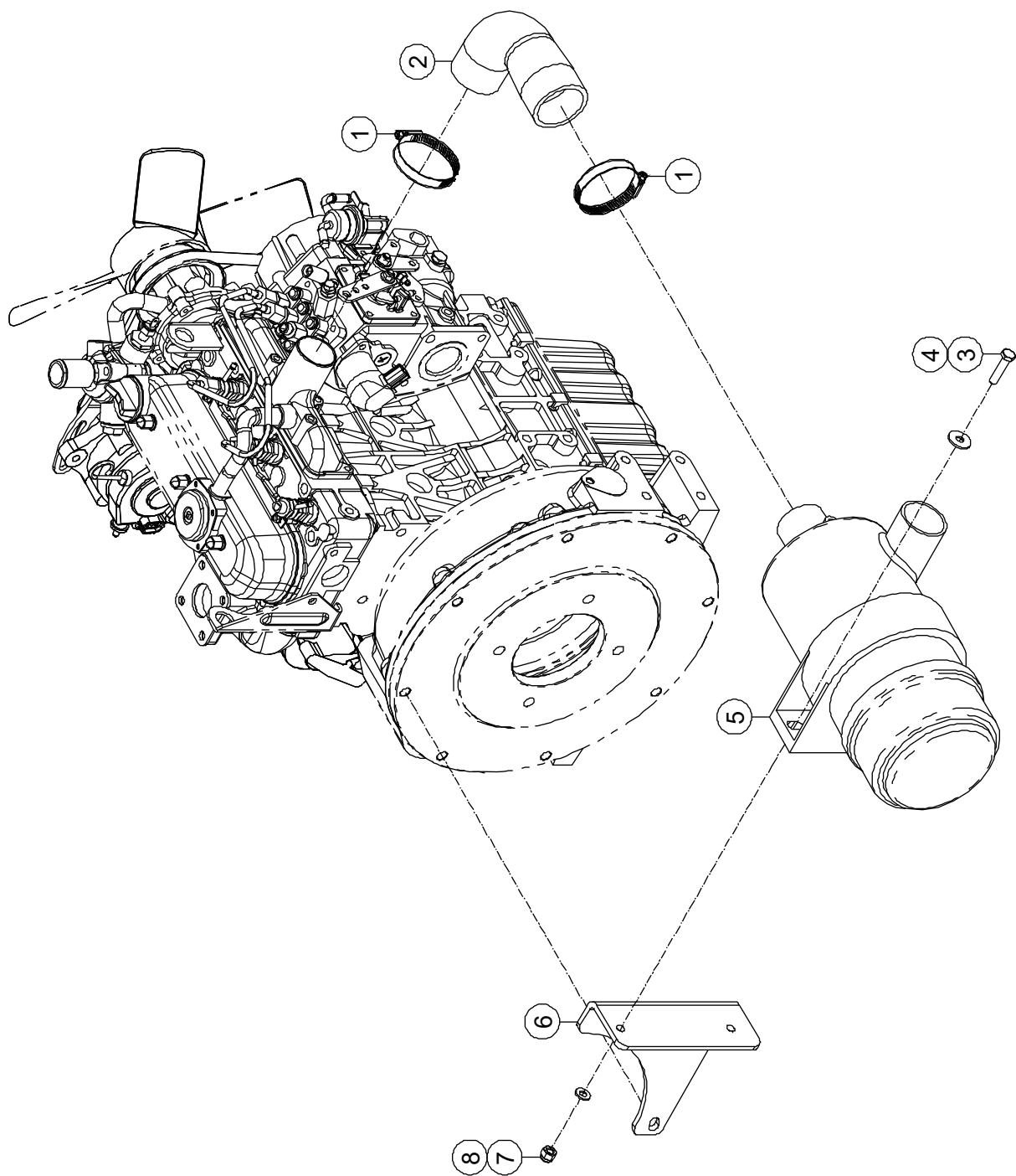
**1-26 Engine Suction System Installations (Kubota Engine)**
