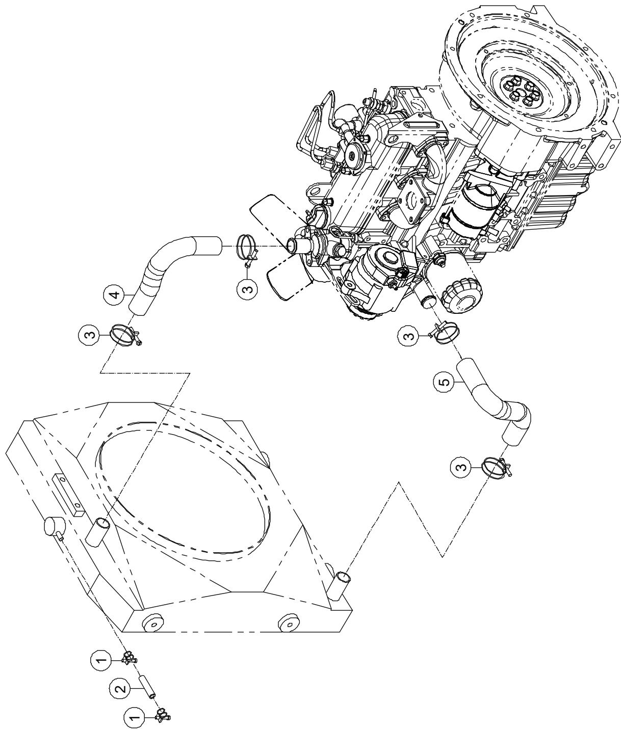
**1-18 Engine Cooling System Installations 2 (Kubota Engine)**
